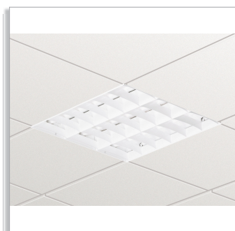
Impala TBS162 recessed luminaire with TL-D fluorescent lamps and an OLC high-gloss high-quality aluminum optic with 3D lamellae, limit 1000 cd (C6-1000cd)
