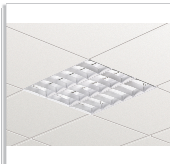
Impala TBS162 recessed luminaire with TL-D fluorescent lamps and a matt high-quality aluminum optic with profiled lamellae (M2)
