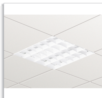
Impala TBS162 recessed luminaire with TL-D fluorescent lamps and a white painted aluminum optic with flat lamellae (L1)
