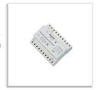
Light regulator for incandescent lamps, high-voltage halogen lamps and low-voltage halogen lamps with electronic transformers. Max. load is 1000 VA, to be used in combination with either a Trios unit, LightMaster Modular (1-10 V) controller or LPS100.
