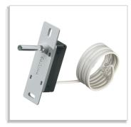
Infrared receiver for remote control of lighting systems and other building-related functions. Only a thin plastic optic protrudes from the ceiling for "invisible" mounting. More infrared receivers can be connected in parallel to cover larger rooms. It is powered from the corresponding controller. Electrical connections with a fixed cable (1 m) with modular plug. Mounting height 2.5 to 4 m. For Trios & LMM systems.
