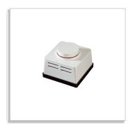
Manual rotary potentiometer with mains switch for surface mounting. In combination with up to 150 Phililps electronic 1-10 V HFR ballasts, electronic light regulators or Trios controllers, it serves to control the light level of fluorescent lamps, halogen lamps or incandescent lamps.
