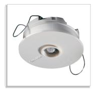
Compact movement detector to be used to expand the detection area for ActiLume and OccuSwitch DALI solutions. The sensor is connected to the DALI bus from the controller (luminaire) and does not require external power. The sensor is suitable for both recessed and surface mounting. Mounting height is between 2.5 and 4 m.
