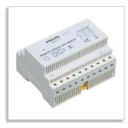
Light regulator for incandescent lamps, high-voltage halogen lamps and low-voltage halogen lamps with conventional transformers. Max. load is 1000 VA, to be used in combination with either a Trios unit, LightMaster Modular (1-10 V) controller or LPS100.
