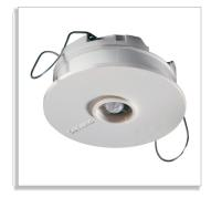
Compact advanced movement detector that features variable delay-to-off via DIP switch and can be part-shaded to limit coverage. The sensor is powered via the additional modular plug-in (RJ12) connector cable that attaches it to a lighting controller. The sensor is suitable for both recessed and surface mounting. Mounting height is between 2.5 m and 4 m. For Trios & LMM systems.
