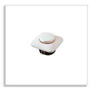
Manual rotary potentiometer with mains switch for recessed mounting. In combination with up to 150 Philips electronic 1-10 V HFR ballasts, electronic light regulators or Trios controllers, it serves to control the light level of fluorescent lamps, halogen lamps or incandescent lamps.
