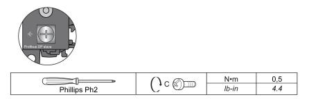
Applying torque above the limit may damage the terminal screw or threads.
