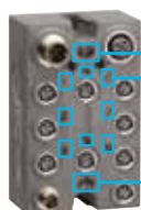
CANopen interface block with digital I/O
