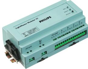
Input unit with 4 sensor interfaces (light sensors, movement detectors and infrared [IR] receivers) and 4 inputs for standard wall switches/emergency test sensors. DIN-rail unit, which is also suitable for use as an installation box, i.e. this unit does not require an outer enclosure.
